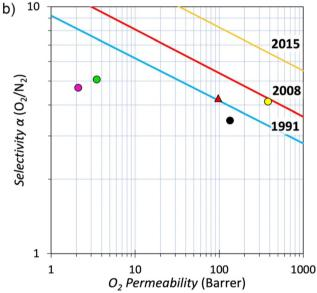
Fig. 5 Robeson plots for a)  $CO_2/CH_4$  and b)  $O_2/N_2$  showing the data for BTFMA-DPE (red) and structurally related polymers TFA-DPE (green) and TFAP-DPE (purple). For comparison, the data points are also provided for PIM-1 <sup>60,61</sup> (yellow) and the much-studied polyimide 6FDA-durene (black). <sup>64</sup>
