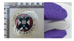
Fig. 4 A robust, optically clear, self-standing film of BTFMA-DPE fabricated from chloroform solution using the techniques of simple solventcasting (5 cm diameter, 100 µm thick).
