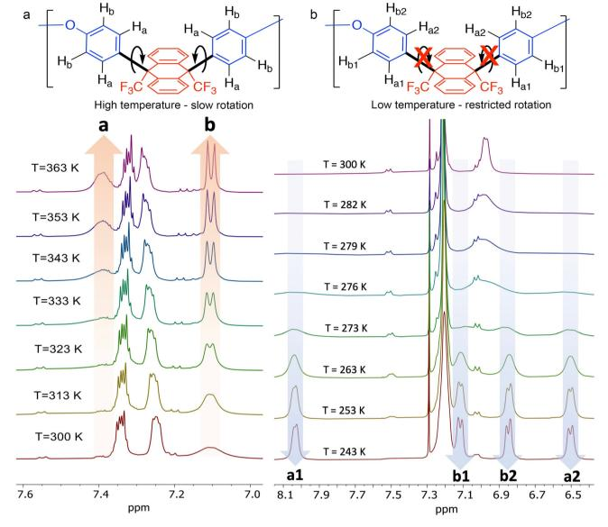
Fig. 3 Variable temperature NMR of polymer BTFMA-DPE acquired in the ranges (a) 300-363 K (in DMF-d<sub>7</sub>) and (b) 243-300 K (in CDCl<sub>3</sub>). Due to hindered rotation of the benzene rings of the DE monomeric unit, the peak for the hydrogens (Ha) adjacent to the new bond only becomes distinct at higher temperatures. At lower temperatures, rotation is frozen so that each of the protons  $H_{a1}$ ,  $H_{a2}$ ,  $H_{b1}$  and  $H_{b2}$  show a distinct peak.
