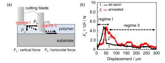
Fig. 4 (a) Schematic representation of SAICAS measurement, showing cutting modes and detecting forces along the directions vertical and horizontal to the interface. (b) Horizontal force ( $F_{\rm h}$ ) profile for the PMMA L & S film before and after annealing, measured in the direction perpendicular to the line pattern.
