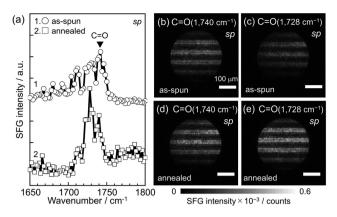
**Fig. 3** (a) SFG spectra in the C=O region with the sp polarization combination for the thin PMMA L&S film before (top) and after (bottom) annealing at 433 K for 24 h. (b-e) SFG images for C=O signals with the sp polarization combination obtained at IR wavenumber of (b and d) 1740 cm<sup>-1</sup> and (c and e) 1728 cm<sup>-1</sup> for the as-spun and annealed films, respectively.
