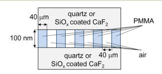
Fig. 1 Side view of a PMMA L & S film
