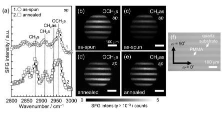
Fig. 2 (a) SFG spectra in the CH region with the sp polarization combination for a thin PMMA L&S film before (top) and after (bottom) annealing at 433 K for 24 h. SFG images for OCH<sub>3s</sub> and CH<sub>2as</sub> signals with the sp polarization combination for the (b and c) as-spun and (d and e) annealed films. (f) A digital microscopic image of the film. The angle formed with the line pattern ( $\omega$ ) is shown.
