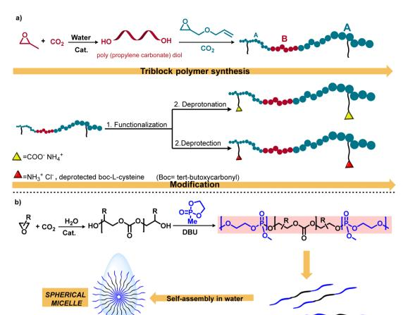
Scheme 3 Sequential approach for the synthesis and functionalization of polycarbonates. (a) Water-mediated polycarbonate synthesis and functionalization to achieve amphiphilic polycarbonates. (b) Illustration of the mechanistic pathway including metal-catalyzed  $CO_2$ /epoxide copolymerization and organocatalytic ring-opening polymerization. (4)
