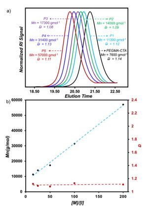
Fig. 3 (a) Representative SEC traces for macro-CTA, and PEGMA<sub>m</sub>-b-PVBzPHT<sub>n</sub> block copolymer: P1-P5; (b) [M]/[I] vs.  $M_n$  of P1-P5.
