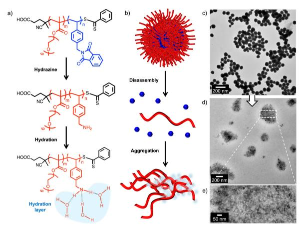
Fig. 6 Schematic representation for disassembly of PEGMA<sub>15</sub>-b-VBzPHT<sub>n</sub> to PEGMA<sub>15</sub>-b-(VBzNH<sub>2</sub>)<sub>n</sub>. (a) Chemical structure, (b) schematic disassembly and aggregation process, (c) representative TEM images for P2 before hydrazine treatment, (d & e) P2 after deprotection and aggregation after hydrazine treatment for 20 h.
