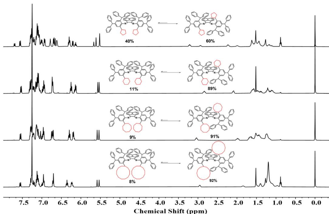
**Fig. 2**  $^1\text{H}$  NMR spectra of ligands  $\text{L}^{\text{C5}}$ – $\text{L}^{\text{C12}}$  at room temperature.
