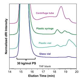
Fig. 5 SEC-MALS chromatograms of a 30 kg mol<sup>-1</sup> PS standard prepared with commonly used plastic laboratory consumable products. All samples were quickly filtered through a 0.22 µm polytetrafluoroethylene (PTFE) syringe filter and added to glass autosampler vials.
