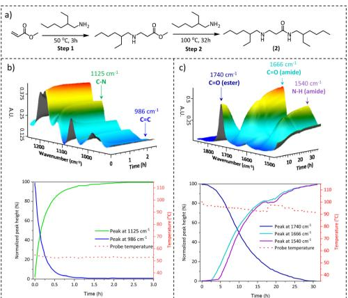
Fig. 3 (a) Synthesis of model compound 2, (b) top: three-dimensional plot of time-resolved ATR-FTIR in the region of 1200 cm<sup>-1</sup> to 900 cm<sup>-1</sup> for the aza-Michael addition step, bottom: plot of the intensity related to the followed peaks *versus* time. (c) Top: three-dimensional plot of time-resolved ATR-FTIR in the region of 1800 cm<sup>-1</sup> to 1300 cm<sup>-1</sup> for the amidation reaction, bottom: plot of the intensity related to the followed peak *versus* time.
