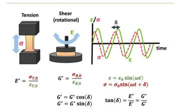
Scheme 12 Schematic of tensile DMA and SAOR, including  $\sigma$  response to sinusoidally applied  $\varepsilon$ , and the complex moduli  $E^*/G^*$  and the storage (E'/G') and loss (E''/G'') moduli. Note that  $\sigma_{T,0}$ ,  $\varepsilon_{T,0}$ ,  $\sigma_{R,0}$ , and  $\varepsilon_{R,0}$  are given in Table 1.
