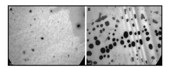
Fig. 6 TEM image acquisition of free (A) T1307-Glu PMs and (B) T1307-Glu/ICG PMs. Scale bar: 0.2 µm. Magnification: 30 000x.
