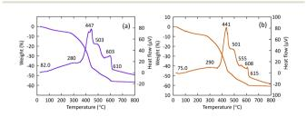
Fig. 2 TG/DTA curves of BNDHP-/LZH, respectively: (a) R-BNDHP-/ LZH (pH 5.0, 60 °C) and (b) S-BNDHP-/LZH (pH 5.0, 60 °C).
