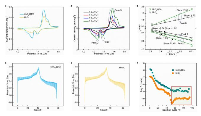
Fig. 4 Electrochemical reaction kinetics of different cathodes. (a) CV curves for  $MnO_2$  and  $MnO_2$ @PA. (b) CV curves of  $MnO_2$ @PA at various sweep rates. (c) The dependence of log (peak current) on log (scan rate) for obtaining b values. Charge/discharge profiles of (d)  $MnO_2$ @PA and (e)  $MnO_2$  during the GITT measurements. (f) The ion diffusion coefficient vs. voltage for  $MnO_2$ @PA and  $MnO_2$  during the 2nd discharge.
