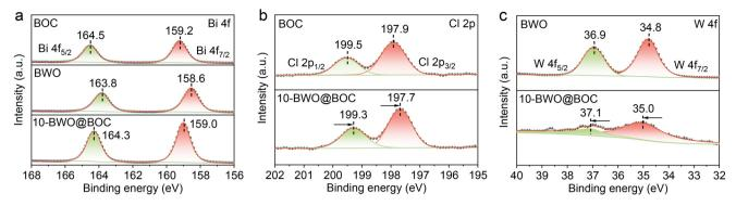
Fig. 3 XPS spectra of (a) Bi 4f, (b) Cl 2p, and (c) W 4f for BOC, 10-BWO@BOC, and BWO.
