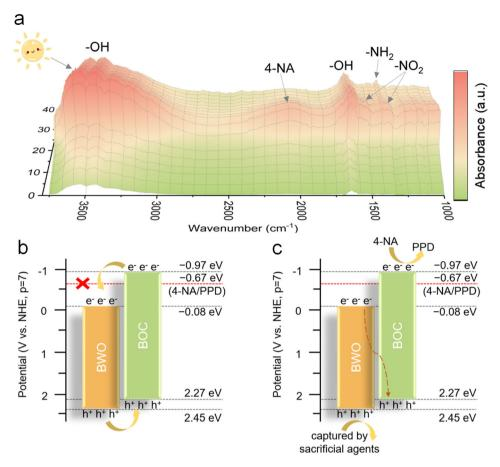
Fig. 8 (a) In situ DRIFTS spectra of 10-BWO@BOC for the adsorption of a mixture of  $H_2O$  and 4-NA for 20 minutes in the dark and under UV-vis light irradiation for another 20 minutes. The proposed charge transfer mechanism of (b) type-II and (c) Z-scheme heterostructures over the 10-BWO@BOC heterostructure for the photocatalytic hydrogenation reaction of 4-NA under UV-vis light irradiation.
