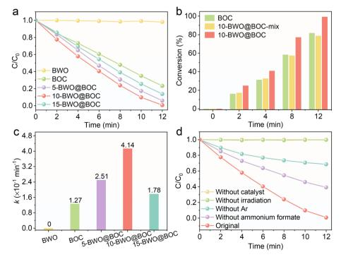
Fig. 4 (a) Photocatalytic performance of 4-NA hydrogenation over the prepared samples under UV-vis light irradiation with ammonium formate as a hole sacrificial agent. (b) Comparison of the 4-NA conversion rates of BOC, 10-BWO@BOC-mix and 10-BWO@BOC. (c) Corresponding apparent reaction rate constants obtained by fitting the pseudo-first-order kinetics model of the prepared samples. (d) Control experiments for the photocatalytic hydrogenation of 4-NA over 10-BWO@BOC.
