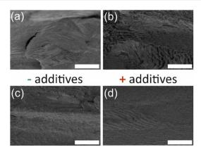
**Fig. 5** SEM images (cross section) of composites prepared from: (a) organosilica precursor and CNC suspension (C-1) and (b) organosilica precursor, CNC suspension and glucose (C-2e); and relevant CNMO films: (c) Et-CNMO-1 and (d) Et-CNMO-2e. Scale bars are 5 μm.
