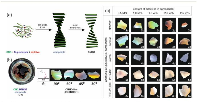
Fig. 1 (a) Preparation of composites and CNMO films. EISA = evaporation-induced self-assembly. (b) Photographs of composites prepared from suspension of CNCs and BTMSE (C-1) and product of hydrolysis - organosilica film (Et-CNMO-1). The photographs are taken at different angles of film position, and ordered by decreasing viewing angle ( $\Theta$ ). (c) Photographs of films of Et-CNMO-2 to Et-CNMO-6 prepared from various composites.
