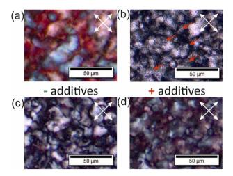
Fig. 4 POM images of composite and CNMO films viewed between crossed polarizers. The samples shown correspond to composites prepared from: (a) organosilica precursor and CNC suspension (C-1) and (b) organosilica precursor, CNC suspension and sucrose (C-3e); and relevant CNMO films: (c) Et-CNMO-1 and (d) Et-CNMO-3e. Red arrows pointing to the non-birefringent regions. Scale bars are 50 μm.
