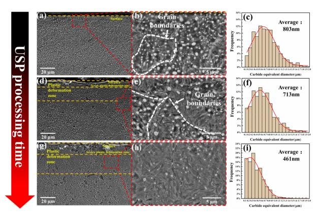
Fig. 2 SEM images of (a) and (b) the as-received GCr15 bearing steel, (d) and (e) the USPed GCr15 bearing steel with the peening duration of 4 min, and (g) and (h) USPed GCr15 bearing steel with the peening duration of 8 min, along the cross-sectional direction. (c), (f) and (i) Statistical analysis of the size of the carbides in the sample with respect to peening durations of 0 min, 4 min and 8 min. The white dashed lines indicate grain boundaries.
