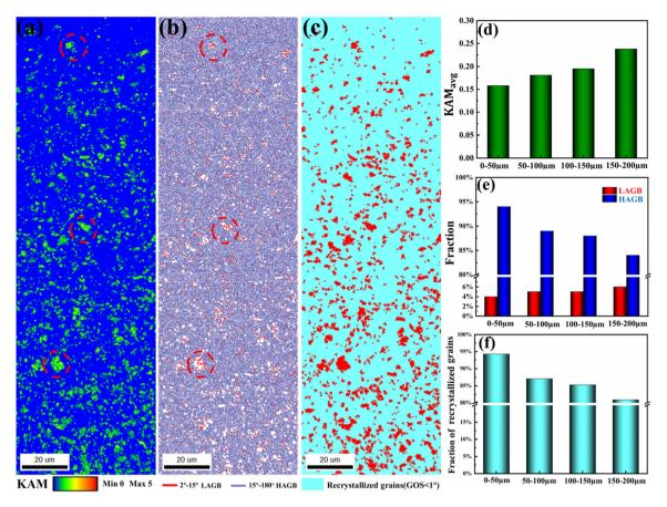
Fig. 12 (a) KAM, (b) grain boundary and (c) GOS mapping of the gradient nanostructured GCr15 bearing steel fabricated by USP with the peening duration of 8 min; statistical analysis of the (d) average value of KAM; (e) fractions of grain boundaries; and (f) fractions of the recrystallized grains of the gradient nanostructured GCr15 bearing steel at different depths.
