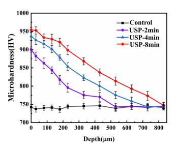
Fig. 9 Microhardness distribution of the AR-GCr15 bearing steel and USPed GCr15 bearing steel with peening durations of 2 min, 4 min and 8 min along their cross-sectional direction.
