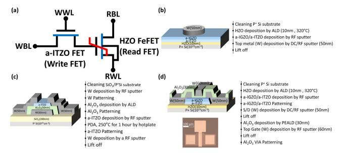
Fig. 2 (a) Layout of the AOS-based 2TOC-FeDRAM cell with schematic device structure and fabrication process flow of (b) W/a-IGZO/a-ITZO/HZO/ P<sup>+</sup> Si MSFM ferroelectric capacitors. (c) The a-ITZO FET as a  $W_{\rm tr}$  and (d) the double gate W/Al<sub>2</sub>O<sub>3</sub>/a-IGZO/a-ITZO FeFET as FE-R<sub>tr</sub>.
