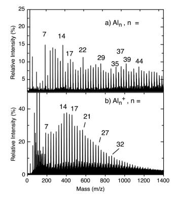
Fig. 1 Typical Al<sub>n</sub> cluster distributions (a) acquired through femtosecond ionization of neutral Al clusters and (b) cation distribution Aln clusters obtained directly through laser ablation. The Al<sub>3</sub>O arises from the high affinity of Al to oxygen. The intensities are normalized to the Al<sup>+</sup> in each respective spectra.
