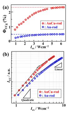
Fig. 5 Excitation intensity  $(I_{ex})$  dependence of (a) upconversion (UC) internal quantum yield ( $\Phi_{\rm UCg}$ ) and (b) UC emission intensity ( $I_{\rm UC}$ ). For comparison, results from a mixture of 50  $\mu$ M AuCu-rod and 20 mM BPFA are also shown.
