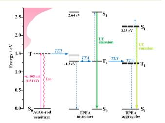
Fig. 6 Schematic energy level diagram of the TTA-UC process in a system comprising the Au-rod sensitizer and 9,10-bis(phenylethynyl) anthracene (BPEA) annihilator monomer and aggregates. TET = triplet energy transfer and TTA = triplet-triplet annihilation.
