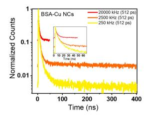
**Fig. 6** The lifetime decay of BSA-Cu NCs with the same time resolution and different repetition rates. The inset image represents the zoomed view of the decay curve within the few nanoseconds time range. The excitation wavelength ( $\lambda_{\rm exc}$ ) used for the measurement is 400 nm.
