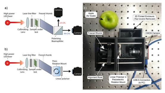
Fig. 1 Schematics of the two- (a) and one-camera (b) circular dichroism imaging systems developed in this work alongside a photograph of the optimised system (c) with a black 3D printed enclosure to block stray light and enable system portability
