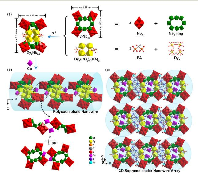
Fig. 1 Structure of 1. (a)  $Dy_8Nb_{64}$  cluster;  $\gamma$ - $Nb_{32}$  cluster;  $Dy_4$  cluster. (b) Representation of the 1D polyoxoanion of 1. Localized schematic of  $Co^{11}$ linking 1 into a nanowire. (c) View of the 3D supramolecular nanowire array. NbO<sub>6</sub> octahedra: red/green; DyO<sub>8</sub> square antiprism: yellow; CoO<sub>6</sub> octahedra: pink.
