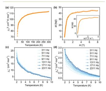
Fig. 2 For 1. (a) Temperature-dependence of  $\chi_{\rm m}T$  in the temperature range of 2-300 K; (b) field-dependence of magnetization at 2 K. Inner: M vs. H/T plots. (c and d) Temperature-dependent behavior of the inphase  $(\chi'_m)$  and out-of-phase  $(\chi''_m)$  in zero static fields at 2–10 K.
