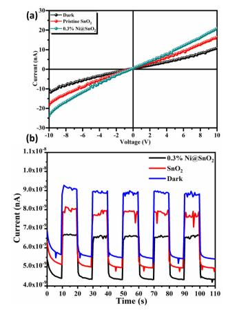
Fig. 13 (a) I-V characteristics and (b) photo-response of pristine SnO<sub>2</sub> and 0.3% Ni@SnO2 photodetectors.
