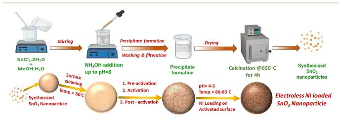
Fig. 1 Process schematic for the synthesis of SnO<sub>2</sub> nanoparticles and their electroless loading with Ni.
