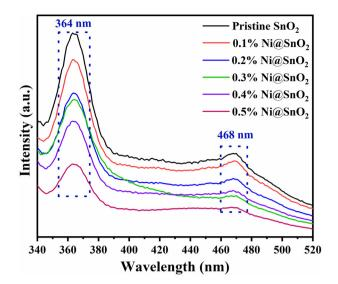
Fig. 6 PL spectra of pristine SnO<sub>2</sub> and Ni@SnO<sub>2</sub> nanostructures.
