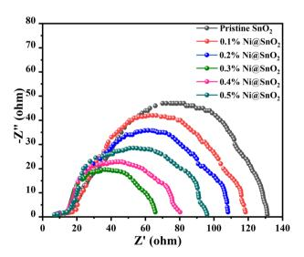
Fig. 12 Nyquist plot for SnO<sub>2</sub> and 0.1 to 0.5% Ni@SnO<sub>2</sub> nanostructures.
