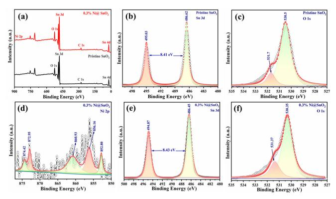
Fig. 3 XPS spectra of pristine  $SnO_2$  and 0.3% Ni@ $SnO_2$  nanostructure samples. (a) Survey scan for both samples, and deconvoluted high-resolution scans corresponding to the elements (b) Sn 3d and (c) O 1s for Pristine  $SnO_2$  and (d) Ni 2p, (e) Sn 3d and (f) O 1s for the 0.3% Ni@ $SnO_2$  nanostructure.
