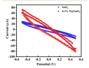
Fig. 14  $\,$  C-V measurement of pristine  ${\rm SnO_2}$  and 0.3% Ni@SnO2 samples.
