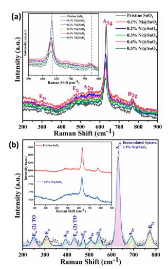
**Fig. 4** Raman spectra of the prepared pristine  $SnO_2$  and  $Ni@SnO_2$  nanostructure in the (a) 200-900 cm<sup>-1</sup> range (inset: 550-800 cm<sup>-1</sup> range) and (b) spectra of  $0.3\%Ni@SnO_2$  nanostructures (inset: 200-900 cm<sup>-1</sup> range for pristine  $SnO_2$  and  $0.3\%Ni@SnO_2$  nanostructure).
