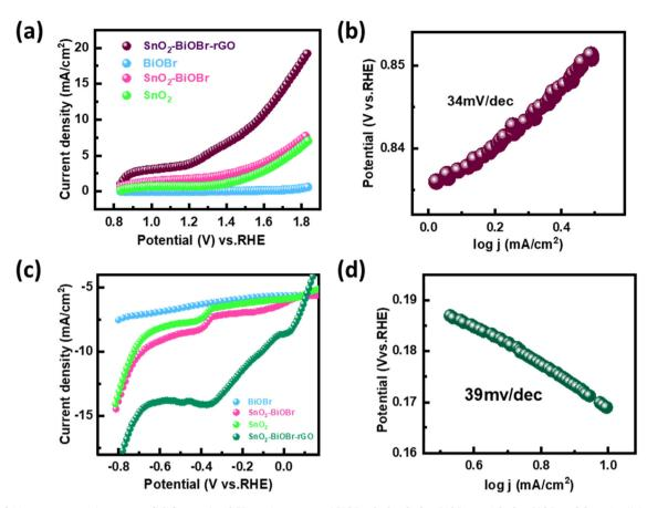
Fig. 12 (a) Linear sweep voltammetry (LSV) scan for OER performance of BiOBr,  $SnO_2$ ,  $SnO_2$ -BiOBr, and  $SnO_2$ -BiOBr-rGO under light irradiation (b) OER Tafel plot for  $SnO_2$ -BiOBr-rGO (c) LSV scan for HER performance of BiOBr,  $SnO_2$ ,  $SnO_2$ -BiOBr and  $SnO_2$ -BiOBr-rGO under light irradiation (d) HER Tafel plot for the  $SnO_2$ -BiOBr-rGO ternary nanocomposite.
