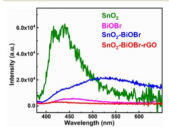
Fig. 6 Photoluminescence spectra of SnO<sub>2</sub>, BiOBr, SnO<sub>2</sub>-BiOBr, and SnO2-BiOBr-rGO.
