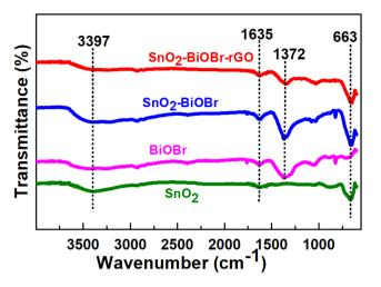
Fig. 2 FTIR spectra for BiOBr, SnO<sub>2</sub>, SnO<sub>2</sub>-BiOBr, and SnO<sub>2</sub>-BiOBrrGO.
