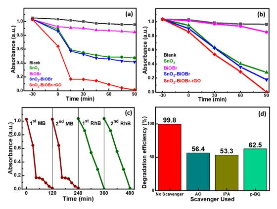
Fig. 8 Kinetics for (a) MB dye and (b) RhB dye degradation using  $SnO_2$ , BiOBr,  $SnO_2$ -BiOBr, and  $SnO_2$ -BiOBr-rGO as photocatalysts. (c) Repeatability test for two cycles for MB and RhB dyes and (d) the effect of adding p-BQ, IPA, and AO as scavengers in RhB dye.
