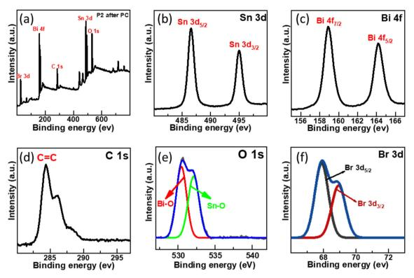
Fig. 11 (a) After photocatalytic treatment the survey scan of SnO<sub>2</sub>-BiOBr-rGO and high-resolution XPS spectrum of (b) Sn 3d, (c) Bi 4f, (d) C 1s, (e) O 1s, (f) Br 3d.
