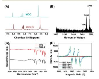
Fig. 1 The structural characterization of MOC and MOC-O nanozymes. (A) The <sup>1</sup>H-NMR spectra of the MOC and MOC-O in DMSO-d<sub>6</sub>. (B) The MALDI-TOF mass spectrum of MOC-O. (C) The FT-IR spectra of the MOC and MOC-O. (D) The EPR curves of the MOC and MOC-O.
