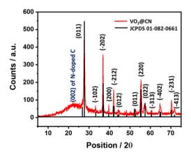
Fig. 2 PXRD pattern of the as-synthesized VO<sub>2</sub>@CN indicating the presence of VO<sub>2</sub> (M) and N-doped carbon.
