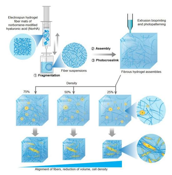
Fig. 6 Schematic of the process of creating reassembled fibrous hydrogels by using fragments of electrospun fiber mats. The study demonstrated that fibers in low-density fibrous assemblies, cells exerting contraction forces could recruit more fibers, leading to increased fiber alignment, greater reduction in hydrogel volume, and higher cell density.
