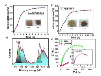
Fig. 4 lodine vapor uptake with time for (a) SBF-BINOL-6; (b) Ag@SBF6. (c) Deconvoluted XPS spectra for iodine in I2@SBF6. (d) The Nyquist plot for SBF-BINOL-6 and I2@SBF6 (inset).
