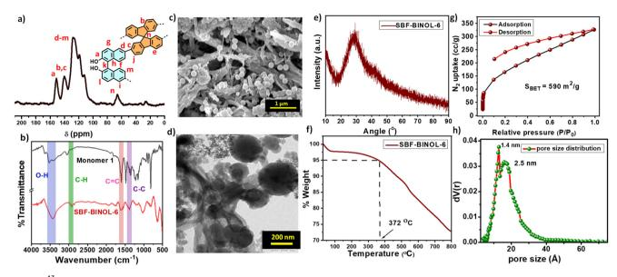
Fig. 1 (a) 13C CP/MAS NMR spectrum, (b) FT-IR spectra along with monomer 1, (c) SEM image, (d) TEM image, (e) PXRD pattern, (f) TGA profile, (g) N<sub>2</sub> adsorption isotherm at 77 K, and (h) pore size distribution of SBF-BINOL-6.
