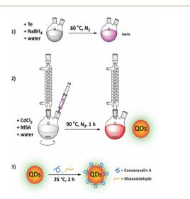
Fig. 1 Illustration of the process of QD synthesis. (1) Generating NaHTe solution at 60 °C under a N<sub>2</sub> atmosphere. (2) Synthesis of QD-MSA. (3) Fabrication of QDs with ConA.
