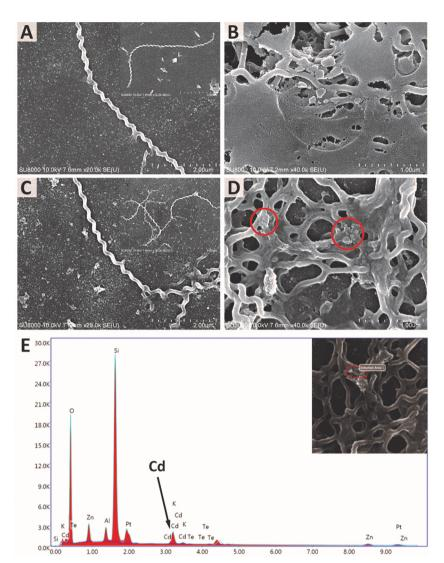
Fig. 9 (A and B) SEM images of *L. santarosai* without and with incubation with ConA-QDs. (C and D) SEM images of *L. interrogans* 53N5 without and with incubation with ConA-QDs. (E) EDX analysis of 53N5 incubated with ConA-QDs. The inset shows the selected area with the observed agglomerate.
