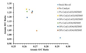
Fig. 7 Van Krevelen diagram for stock and upgraded bio-oils obtained over all the synthesized LiCoO<sub>2</sub> and Co<sub>3</sub>O<sub>4</sub> loaded HZSM-5 catalysts.
