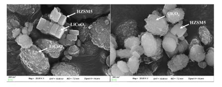
Fig. 5 FESEM micrographs of LiCoO $_2$  and Co $_3$ O $_4$  loaded HZSM-5 catalysts.
