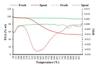
Fig. 8  $\,$  TG and derivative TG plots of fresh and spent 10% Co (LiCoO<sub>2</sub>)/HZSM-5 catalysts (cycle I).
