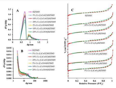
Fig. 2  $N_2$  Ads/Des isotherms (C) and pore size distributions (micropores (A) and mesopores (B)) of all the synthesized LiCoO<sub>2</sub> and Co<sub>3</sub>O<sub>4</sub> loaded HZSM-5 catalysts.
