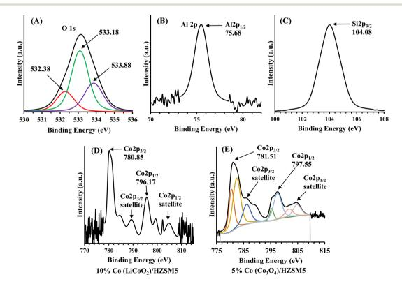
Fig. 3 XPS spectrum of (A) O (1s), (B) Al (2p), (C) Si (2p), (D) Co (2p) of 10% Co (LiCoO<sub>2</sub>)/HZSM-5 and (E) Co (2p) of the 5% Co (Co<sub>3</sub>O<sub>4</sub>)/HZSM-5 catalyst.
