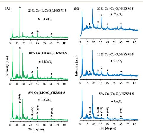
Fig. 1 (a) XRD patterns of 5%-20% Co(LiCoO<sub>2</sub>)/HZSM-5 catalysts. (b) XRD patterns of 5%-20% Co(Co<sub>3</sub>O<sub>4</sub>)/HZSM-5 catalysts.
