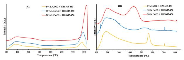
Fig. 4 NH<sub>3</sub>-TPD profiles of all the synthesized (A) LiCoO<sub>2</sub> and (B) Co<sub>3</sub>O<sub>4</sub> loaded HZSM-5 catalysts.
