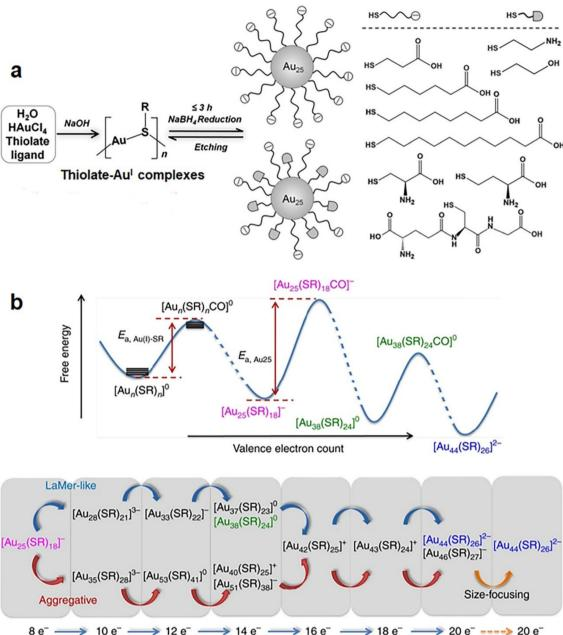
Fig. 4 (a) Schematic illustration of the NaOH-mediated NaBH<sub>4</sub> reduction method for the synthesis of  $[Au_{25}(SR)_{18}]^-$  NCs with a broad library of thiolate ligands (shown in right). Reproduced from ref. 67 with permission from John Wiley and Sons, copyright 2014. (b) Schematic illustration of the CO-mediated size growth reaction from  $[Au_{25}(SR)_{18}]^-$  to  $[Au_{44}(SR)_{26}]^{2-}$ . Reproduced from ref. 69 with permission from Nature, copyright 2017.
