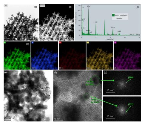
Fig. 3 (a) and (b) TEM images of (Aq,Au)/Mo-BiVO<sub>4</sub> PC340 films and (c) the corresponding local EDX spectrum and (d) Bi, V, O, Mo, Aq and Au elemental maps obtained from (e and f) higher magnification TEM images of (Ag,Au)/Mo-BiVO<sub>4</sub> and (g) the FFT patterns of the encircled areas in (f), where individual Ag and Au NPs can be identified.
