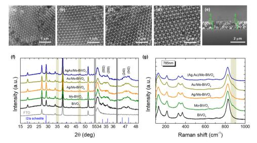
Fig. 2 Plan view SEM images for (a) PC239, (b) PC287, (c) PC340, (d) PC418, and cross section for (e) PC340 inverse opal films. (f) XRD patterns and (g) Raman spectra of Aq, Au-modified Mo-BiVO<sub>4</sub> PC340 films compared to the pristine Mo-doped and undoped BiVO<sub>4</sub>. The XRD patterns of the FTO substrate and the ms phase (JCPDS 014-0688) are also displayed, while the right panels in (f) depict in detail the shaded areas of the XRD patterns.
