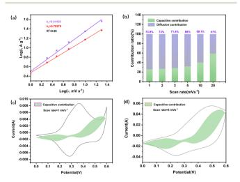
Fig. 8 (a) Kinetic characteristics and reaction mechanism of CoNi<sub>0.5</sub>-MOF/CC electrode; (b) the capacitive contribution of CoNi<sub>0.5</sub>-MOF/CC at different scan rates; (c and d) the capacitive contribution at 1 mV s<sup>-1</sup> and 5 mV  $s^{-1}$ .
