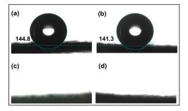
Fig. 2 Hydrophilicity test of CC after different pretreatment processes: (a) original CC; (b) treated with KOH; (c) treated with HNO<sub>3</sub>/H<sub>2</sub>SO<sub>4</sub>/ KMnO<sub>4</sub> mixture; (d) treated with H<sub>2</sub>O<sub>2</sub>.
