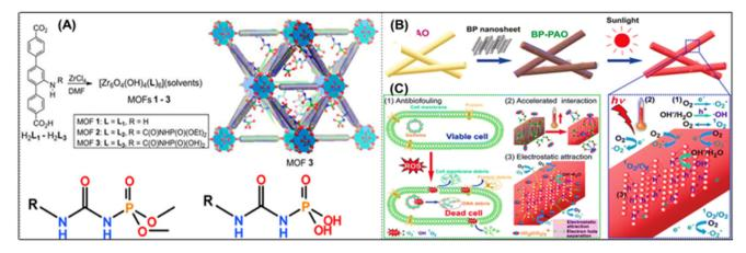
Fig. 5 (A) Diagram illustrating the combination of 1–3. (Bottom) Right and left 1 and 2 have orthogonal functionalities. (B) Diagrammatic representation of the BP-PAO fibre preparation process. (C) Mechanism of the BP-PAO fiber uranium absorption and antifouling. 122
