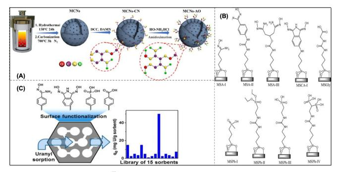
Fig. 7 (A) The MCNs-AO preparation scheme. (B) Mesoporous silica sorbents with organo functionalization for removing U from both artificial seawater and water. (C) Adsorbents made of functionalized mesoporous carbon. (40)
