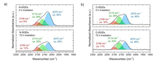
Fig. 4 Deconvoluted FT-IR spectra of (a) N-SiQDs and (b) O-SiQDs as prepared (top) and following 72 h UV irradiation (bottom) spanning the  $SiH_x$  stretching region and deconvoluted to show the contributions from  $SiH_3$  (red),  $SiH_2$  (green), and SiH (blue) components. In general, a decrease in the  $SiH_x$  contribution is noted after irradiation.
