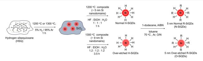
Scheme 1 Preparation of 'normal' and 'over-etched' dodecyl-functionalized SiQDs. Freestanding H-SiQDs were liberated from HF-etching of thermally-processed HSQ, followed by radical-initiated hydrosilylation with 1-dodecene.
