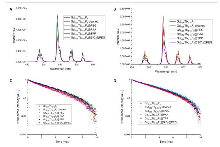
Fig. 5 (A) Luminescence spectra of the various surface-modified  $Gd_{0.9}Tb_{0.1}F_3$  systems in  $H_2O$ , with excitation at 273 nm. (B) Luminescence spectra of the various surface-modified  $Gd_{0.9}Tb_{0.1}F_3$  systems in  $D_2O$ , with excitation at 273 nm. (C) Lifetime decay of the colloidal suspension of  $Gd_{0.9}Tb_{0.1}F_3$ systems in  $H_2O$ . (D) Lifetime decay of the colloidal suspension of  $Gd_{0.9}Tb_{0.1}F_3$  systems in  $D_2O$ .
