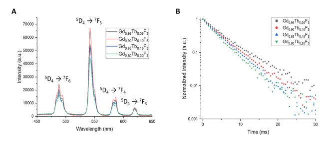
Fig. 2 (A) Luminescence spectra of the various NC compositions after excitation at 273 nm. (B) Lifetime decay measurements after excitation at 273 nm.
