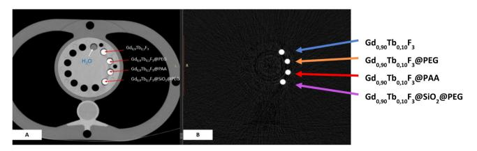
Fig. 7 (A) Conventional SPCCT imaging of a phantom containing colloidal suspensions of normal, PEG modified, PAA modified and SiO<sub>2</sub>@PEG modified NCs in water (0.5 M). (B) Same phantom with color gadolinium K-edge imaging using SPCCT.
