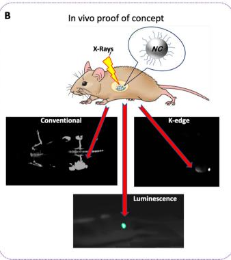
Scheme 1 Conceptual advance of this work with (A). Demonstration of the spectral photon-counting scanner (conventional and color gadolinium K-edge)/luminescence imaging of optimized contrast agents, and (B). In vivo proof of concept for multimodal imaging.
