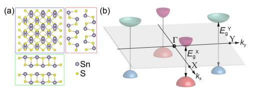
Fig. 1 Crystal structure and band edges of orthorhombic SnS. (a) Crystal structure of SnS (space group Pnma). Red, green, and blue boxes show views along [100], [010], and [001] axes. (b) Schematic illustration of the valence- and conduction band edges of SnS along  $k_x$  and  $k_y$  reciprocal space axes, with bandgaps  $E_q^X$  and  $E_q^Y$  of the non-degenerate X- and Y-valleys, respectively.
