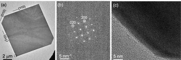
Fig. 2 Structure and morphology of homogeneous SnS flakes. (a) TEM image of an entire SnS flake (side length 9.4 μm). (b) Nanobeam electron diffraction pattern of the flake, identifying the major side facets as {110} facets. (c) High-resolution TEM image showing SnS lattice fringes throughout the flake up to the free surface.
