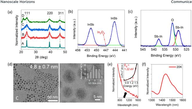
Fig. 1 (a) Powder XRD patterns of the products prepared with different centrifugation processes; a detailed scheme has been added in Scheme S1 (see ESI†). XPS spectra in (b) In 3d and (c) Sb 3d core levels of sample C, fitted with a Gaussian function. (d) HR-TEM image of sample C with the size distribution profile shown in the inset. (e) Room-temperature NIR absorption spectrum of sample C dispersed in TCE. (f) PL spectra of sample C at a temperature of 20 K.
