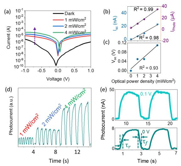
Fig. 4 (a) Logarithmic I-V characteristics of the QPD at 1100 nm with different optical light intensities. Optical illumination intensity-dependent (b) I<sub>SC</sub>,  $I_{\rm photo}$  (-1 V) and (c)  $V_{\rm oc}$  values (linear fit) of the QPD. (d) Photoresponse of the QPD at different light intensities of 1100 nm light. (e) Photoresponse of the QPD at 0 and 0.1 V.
