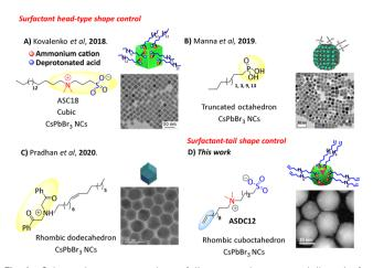
Fig. 1 Schematic representation of literature documented ligands for the synthesis of CsPbBr<sub>3</sub> NCs and their respective NC morphologies. (A) Adapted with permission from ref. 8. Copyright 2018 American Chemical Society. (B). Adapted with permission from ref. 9. Copyright 2019 American Chemical Society. (C). Adapted with permission from ref. 10. Copyright 2020 American Chemical Society. (D) Our work, surfactant-tail control of CsPbBrz NCs morphology.
