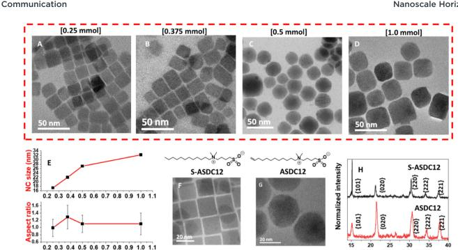
Fig. 4 (A)-(D) TEM analysis of CsPbBr<sub>3</sub> NCs synthesized at different ASDC12 concentrations; (E) changes in the size and NC ratio of CsPbBr<sub>3</sub> NCs at different ASDC12 concentrations; (F) and (G) Chemical structure of S-ASDC12 and ASDC12 and TEM images of their respective NCs (G). (H) PXRD patterns of NCs capped with S-ASDC12 (gray) and ASDC12 (red).
