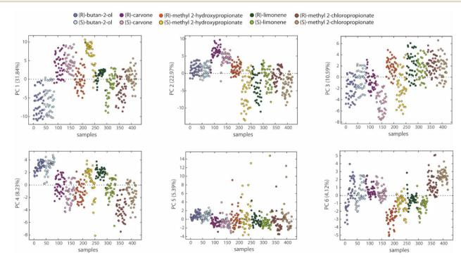
Results of PCA applied to sensors data: scores plot of samples vs. principal components from PC1 to PC6 for all tested analytes.
