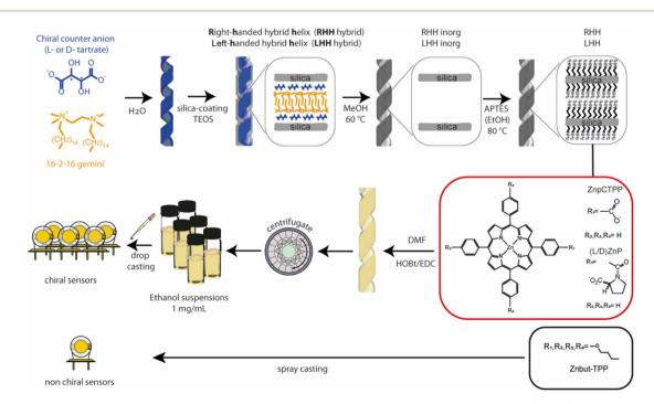
Fig. 1 Schematic representation of synthetic steps of chiral nano helices, porphyrin receptors utilized, (b) and (L)ZnP and ZnpCTPP, and deposition steps on the QMBs surface.
