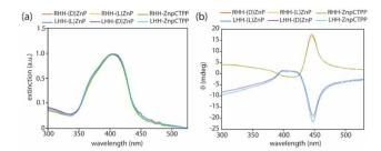
Fig. 2 (a) UV-Vis and (b) CD spectra of porphyrins functionalized chiral nanohelices drop-casted on quartz slides.
