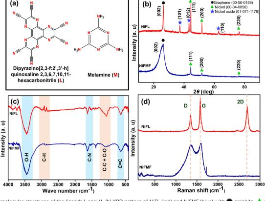
Fig. 1 (a) The molecular structures of the ligands L and M, (b) XRD pattern of NiFL (red) and NiFMF (blue) with 🌑 graphite, 🛕 nickel and 🤸 nickel oxide, (c) IR spectra of NiFL (red) and NiFMF (blue), and (d) Raman spectra of NiFL (red) and NiFMF (blue).
