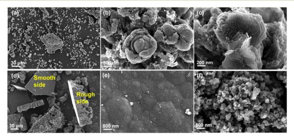
Fig. 3 FESEM images of NiFL and NiFMF. Images (a), (b) and (c) correspond to NiFL, and images (d), (e), and (f) correspond to NiFMF at comparable magnifications. Images e and f show the smoother and rougher surfaces of NiFMF, respectively.
