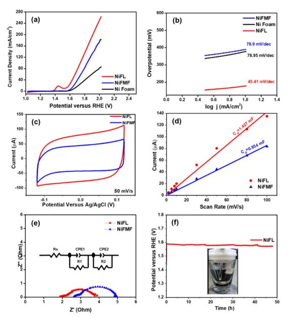
Fig. 6 (a) Linear sweep voltammetry (LSV) curves at 5 mV s $^{-1}$ , (b) corresponding Tafel plot, (c) comparison of CVs for 50 mV s $^{-1}$  with (d)  $C_{\rm all}$  calculation, (e) Nyquist plots of different electrocatalysts at 0.6 V *versus* Ag/AgCl in 1 M KOH solution, (f) chronopotentiometric stability test of NiFL at 20 mA cm $^{-2}$  for 48 h.
