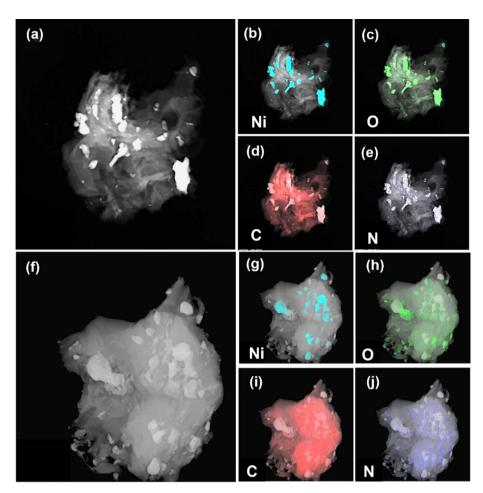
Fig. 5 TEM image and elemental distribution of NiFL (a-e) and NiFMF (f-j). The signals corresponding to the elements are light blue (Ni), green (O), red (C), and dark blue (N).
