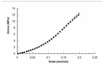
Fig. 3 Typical stress-strain curves obtained for 3D AM PCL ( $\bullet$ ) and GL-coated PCL ( $\triangle$ ) scaffolds (rate of 1 mm min<sup>-1</sup> and final strain of 20%).
