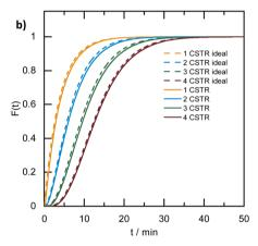
Fig. 3 RTD profiles of the CSTR cascade (for a one to four CSTR configuration) (a) E(t) and (b) F(t) (flow rate: 3 mL min<sup>-1</sup>, stirring speed: 650 rpm, solid lines: experimental RTD profiles, dashed lines: profiles based on the ideal CSTRs in series model).
