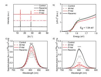
Fig. 2 Effect of helical modulation on the properties of FA<sub>0.97</sub>- $MA_{0.03}Pb(I_{0.97}Br_{0.03})_3$  perovskite films. (a) XRD patterns and (b) the corresponding Tauc plots. (c and d) Absolute intensity steady-state PL for control (grey) and modulated (red, black) films on microscope glass in the absence (c) and presence (d) of HTM (spiro-OMeTAD). Numbers represent PLQY and quasi-Fermi level splitting (ΔE<sub>F</sub>; Table S6†).<sup>40</sup> TRPL data is shown in Fig. S19-S21.†
