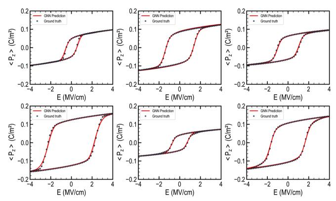
Fig. 6 Ferroelectric hysteresis prediction by the GNN framework. Illustrations of ferroelectric hysteresis predictions are presented alongside their corresponding ground truths from the testing dataset. The model predictions are displayed with solid lines for the sake of clarity, despite the fact that they are composed of 100 discrete points. The ground truths are represented by discrete data points. The model's predictions accurately capture various types of hysteresis shapes.
