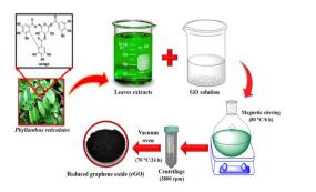
Fig. 6 Green reduction of graphene oxide (GO) using an aqueous leaves extract.
