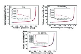
Fig. 13 Nitrogen-adsorption/desorption isotherms and corresponding pore size distribution of (a) pure WO<sub>3</sub>, (b) 1% rGO/WO<sub>3</sub> and (c) 5% rGO/WO<sub>3</sub>. This figure has been reproduced from ref. 247 with permission from the Royal Society of Chemistry, Copyright 2019.
