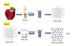
Fig. 9 Synthesis of GO and rGO/ZnO NCs via hydrothermal method.
