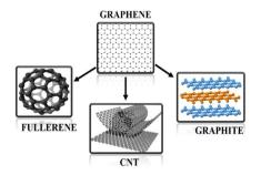
Fig. 1 Graphene is a 2D building block for carbonaceous materials of all other dimensions. It can be wrapped into 0D buckyballs, rolled into 1D nanotubes or stacked into 3D graphite.
