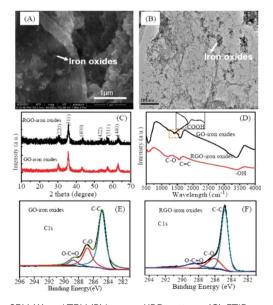
Fig. 10 SEM (A) and TEM (B) images, XRD patterns (C), FTIR spectra (D), and high-resolution C 1s (E and F) XPS of GO-Fe $_3$ O $_4$  NC and rGO-Fe $_3$ O $_4$  NC hybrid materials. This figure has been reproduced from ref. 244 with permission from the Royal Society of Chemistry, Copyright 2012.
