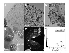
Fig. 12 TEM analysis of graphene/Mn $_3O_4$  NCs: products prepared at reaction times of 4 h (a), 8 h (b), and 16 h (c); HRTEM image of attached Mn $_3O_4$  NPs (d) and corresponding SAED pattern (e); and (f) EDS pattern of Mn $_3O_4$  NPs. Reproduced with the permission from ref. 246. Copyright 2017, the Royal Society of Chemistry.
