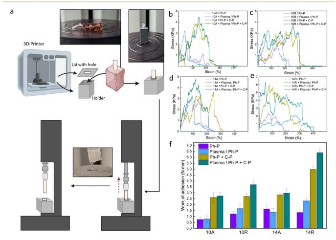
Fig. 3 Fiber pull-out test. (a) Scheme of the customized 3D-printed holder for the nanoplatforms and the test steps. (b–e) Stress–strain curves for (b) PCL10A, (c) PCL10A, (d) PCL14A, (e) PCL14R paired with hydrogel in all the conditions. (f) Nanoplatforms' toughness, measured by calculating the work per unit volume for each group set as an indicative value of the adhesion and incorporation of interfaces.
