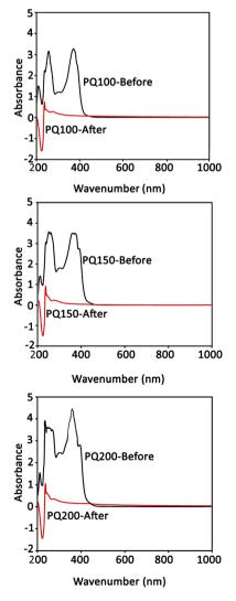
Fig. 3 The quercetin UV absorption spectra of the loading media (ethanol) before and after the loading procedure.
