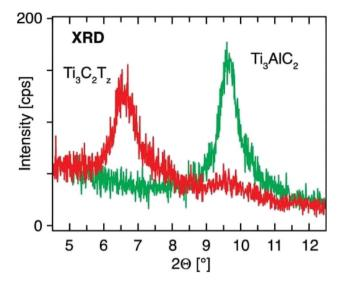
Fig. 7 XRD image of Ti<sub>3</sub>AlC<sub>2</sub> and Ti<sub>3</sub>C<sub>2</sub>T<sub>x</sub>. The diffractogram shows the Ti<sub>3</sub>AlC<sub>2</sub> film at 9.65 and the Ti<sub>3</sub>C<sub>2</sub>T<sub>x</sub> film at 6.60.<sup>45</sup>
