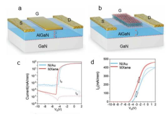
Fig. 18 GaN HEMT schematic diagrams with either  $Ti_3C_2T_x$  or (a) Ni/Au or (b) the gate electrodes. (c) The Ni/Au- and MXene-gate GaN HEMTs'  $I_G$ curves and logarithmic-scale transfer curves. (d) GaN HEMT dual-sweep transfer curves on a linear scale (copyright 2023 John Wiley and Sons).
