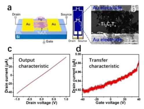
Fig. 11 The  $Ti_3C_2T_x$  FET sensor's schematic structure is shown in (a). (b) A picture of the FET sensor electrodes and a SEM image of the  $Ti_3C_2T_x$  nanosheets joining the nearby gold finger electrodes. (c) A  $Ti_3C_2T_x$  FET device's output characteristics and (d) transfer characteristics.
