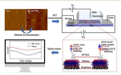
Fig. 14 FET circuit and illustration of the antibody-antigen sensing mechanism and change in drain source current.<sup>17</sup>
