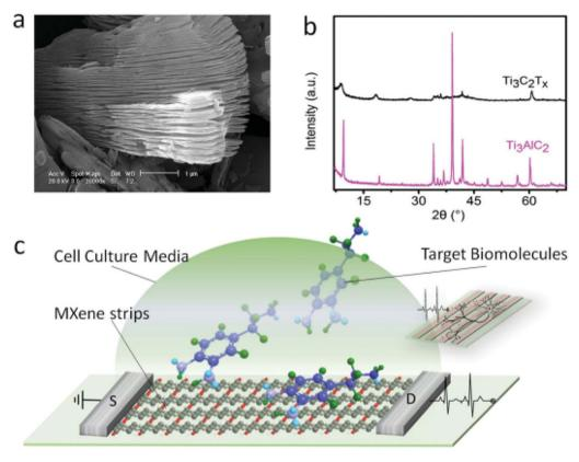
Fig. 17 Characterization of bulk MXenes. (a) SEM image of the multilayer structured MXene. (b) XRD patterns of the transition from  $Ti_3AlC_2$  to  $Ti_3C_2T_X$ . (c) Schematic of a biosensing device based on MXene field effect transistors (copyright 2016 John Wiley and Sons).<sup>151</sup>
