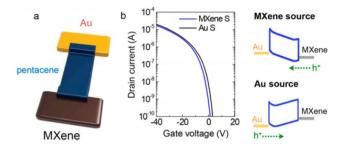
Fig. 13 (a) A schematic depiction of MXene/pentacene/Au. (b) P-type pentacene OFET transfer characteristics with a Au source electrode (black) and MXene source electrode (blue) are shown.<sup>145</sup>
