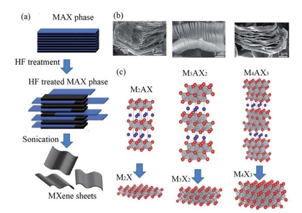
Fig. 1 (a) Three distinct MXene (non-terminated) structures were initially reported:  $M_2X$ ,  $M_3X_2$ , and  $M_4X_3$ . (b) SEM pictures of  $Ti_2AlC_2$ , and  $Ti_4AlC_3$  (from right to left) after HF treatment. (c) Illustration of the synthesis of MXenes from MAX phases in a schematic form.
