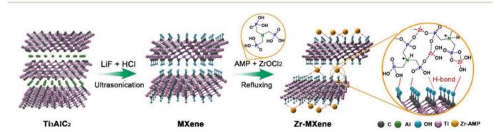
Fig. 3 Scheme for the Zr-MXene preparation.<sup>37</sup>
