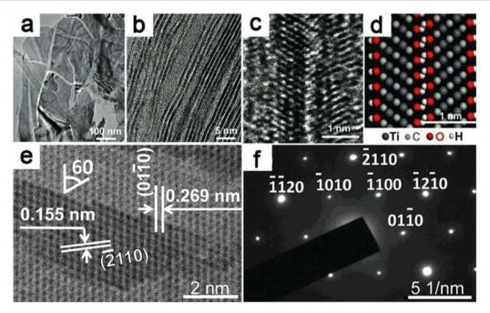
Fig. 10 SAED and TEM imaging of MXenes. (a) A TEM picture of exfoliated Ti-C-O-F 2D nanosheets. (b) MXene sheets with one or two layers. (c) HRTEM picture of bilayer  $Ti_3C_2(OH)_xF_V(d)$  its atomistic model of the layer structure (e) HRTEM image of multilayered MXene and (f) MXene's SAED pattern.⁵⁴
