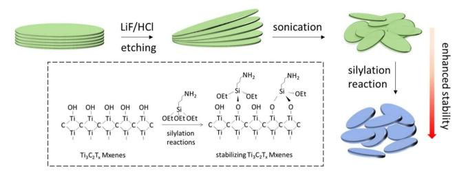
Selective etching and sonication of MXenes with LiF/HCl (copyright 2019 Elsevier)
