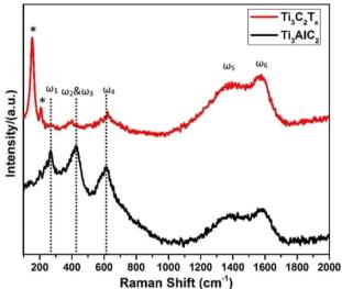
Fig. 5 The Raman spectra exhibit distinctive features for both Ti<sub>3</sub>AlC<sub>2</sub> MAX powder and Ti<sub>3</sub>C<sub>2</sub>T<sub>x</sub> MXene. Peaks labeled with "\*" specifically correspond to the out-of-plane vibrations of titanium (Ti) and carbon (C) atoms in the structure.
