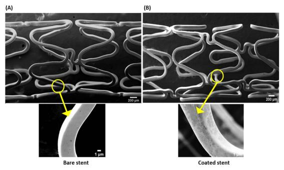
Fig. 1 Scanning electron micrographs of surface morphologies of (A) bare (uncoated) and (B) coated stents. Magnifications: upper panels,  $25 \times (\text{scale}, 200 \ \mu\text{m})$ ; lower panels,  $400 \times (\text{scale}, 1 \ \mu\text{m})$ .
