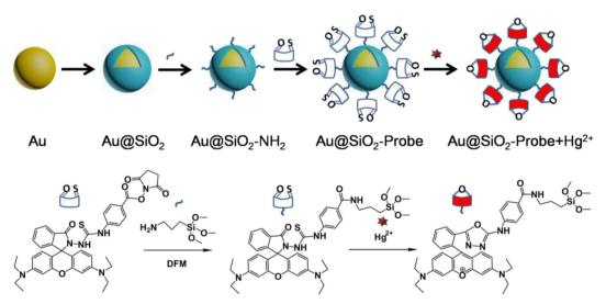
Scheme 1 Schematic illustration of the preparation flow for the fluorophore-labeled Au@SiO<sub>2</sub> NP probe and its detection mechanism for Hg<sup>2+</sup> ions.
