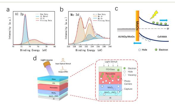
Fig. 2 XPS studies and mechanisms of CsFAMA optoelectronic synapses. XPS spectra of (a) Al 2p and (b) Mo 3d. (c) Energy band diagram of the Al/MoO<sub>3</sub>/CsFAMA/ITO device under an optical stimulus. (d) Schematic of the device and the microscopic operation mechanism.
